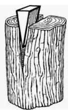
When you insert a screw or any other body into the wood, you generate pressure inside the wood. The wood fibers are pushed away from the area of the Screw. It is even more crucial when screwing close to the edge of the board, where the ability to absorb the pressure is reduced dramatically.
